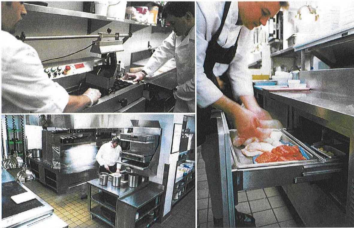
Clockwise from far right: Under-the-counter refrigerated drawers keep chilled ingredients close at hand for executive sous chef Tod Wentz and the rest of the brigade. 85 foot-candle illumination makes Lacroix's kitchen a well lit workspace. In the Chocolate Laboratory, pastry chef Fredrick Ortega oversees another batch of Lacroix's handmade chocolates as they emerge from the enrober.
